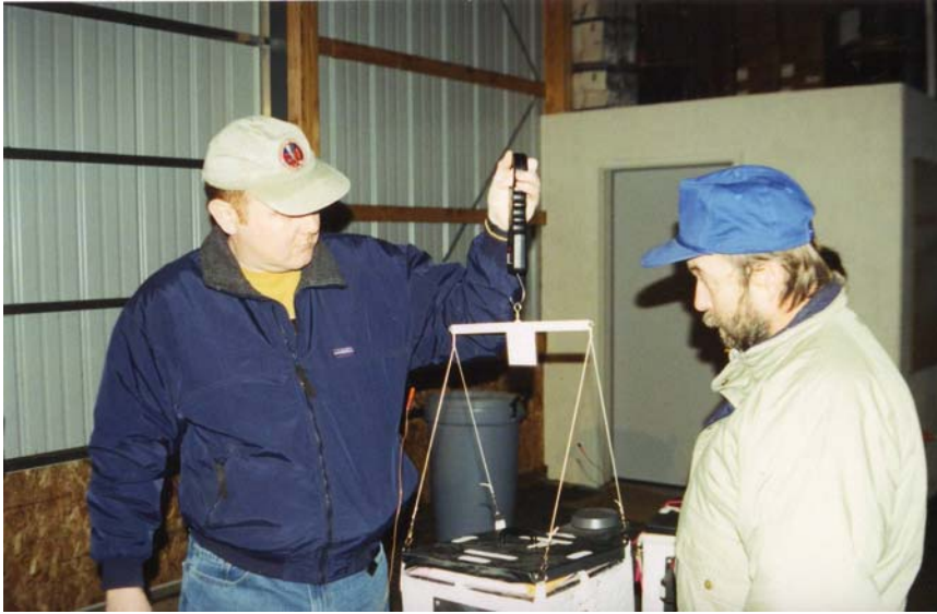
Weighing Frame - Mark Conner (N9XTN) and Dan Miller (KC7SLC) weighing a module of a near spacecraft
