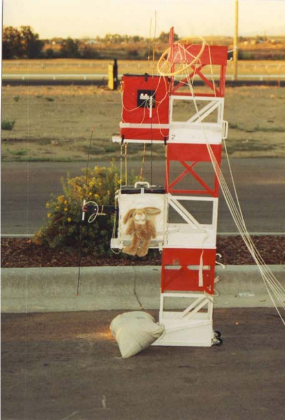
The Launch Tower – Holding the assembled near spacecraft. The modules and parachute are all linked up. Mr. Bunny will skydive from 50,000 feet on this mission.
