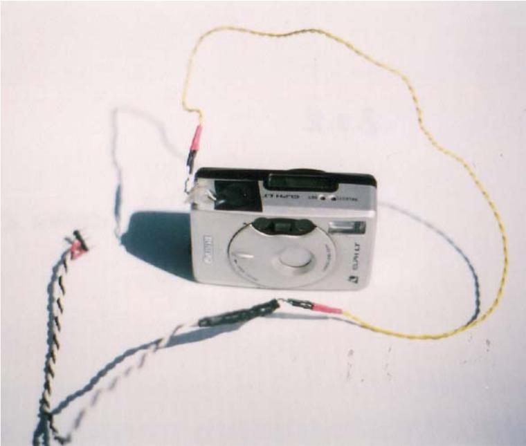
*Modified Camera – With wires twisted*
