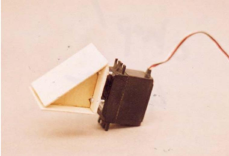
*Mirror Wedge Attached to the Servo*
