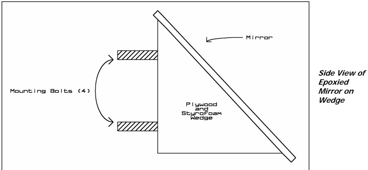
Center and epoxy the mirror to the diagonal face of the wedge with the aluminized face up.
