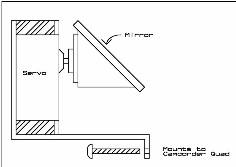
**Rotating Mirror** – Mounts to camcorder quad.
