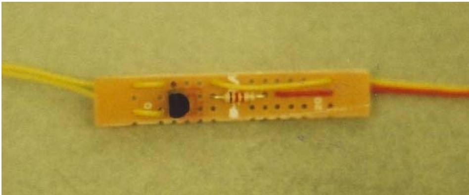
**Camera Transistor Switch – Built on perf board**
