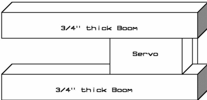
**Booms Holding Servo** – Two 3/4" thick Styrofoam booms support the servo.
