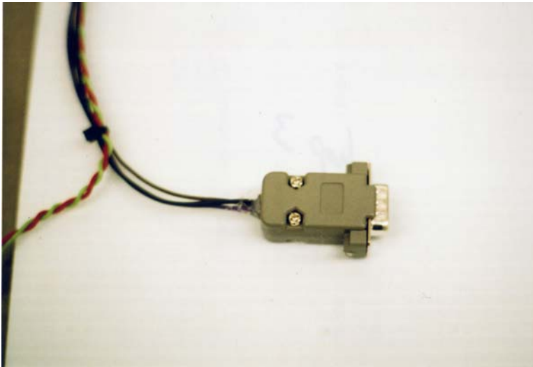
DB-9 Connector – Housing for GPS DB-9 connector. Interior volume is filled with hot glue.
