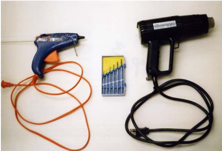
Tools – Hot glue gun, jeweler's screwdrivers, and hot air gun.
