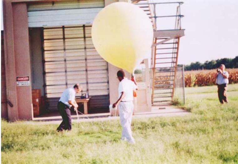
***Out to Launch*** - A meteorologist from the N.W.S. getting ready to release a radiosonde.
