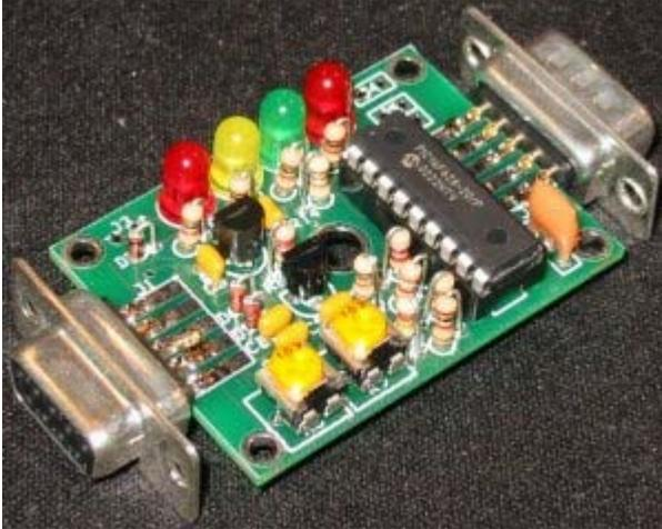
*Tiny Trak III* – A completely assembled Tiny Trak. Yours will be similar. (Photo by Byon Garrabrant)
