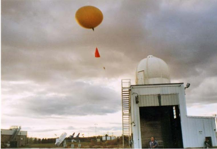
***Up and Away** - A radiosonde is released in front of the filling building.*
