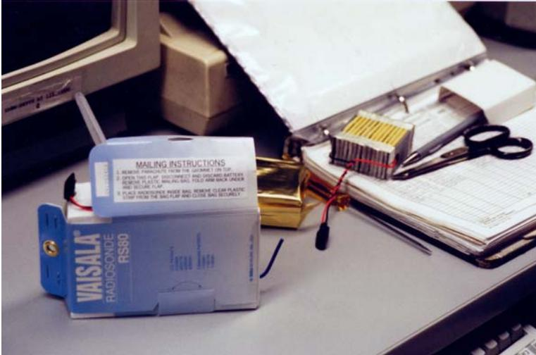
*Sonde on Desk - The Vaisala Radiosonde being prepped for launch. The battery is on the notebook.*
