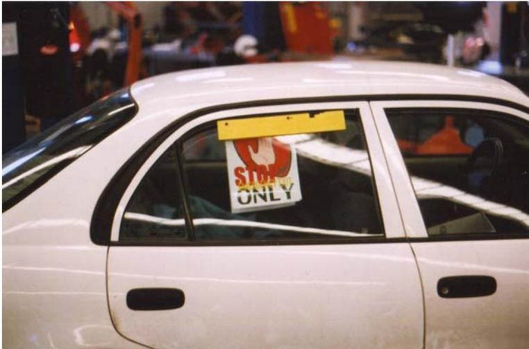
*Example of Window Pass-Through on Vehicle – Sign reads "STOP Emergency Exit Only"*
