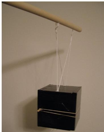
FIGURE 4-5. A BalloonSat undergoing a shake test.
