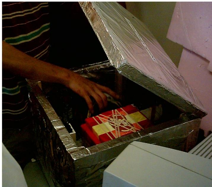
**FIGURE 4-2. Loading a BalloonSat into a thermal test chamber.**
