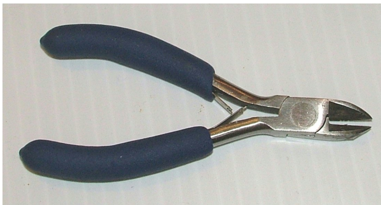
Figure 2. A small pair of wire cutters lets you clip wires closer to the surface of the robot controller
