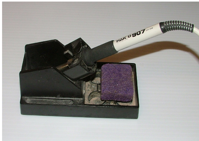
Figure 4. The soldering iron in its stand and with its sponge. Never lay a hot soldering iron on the table, always use a stand. And always keep the sponge damp.
