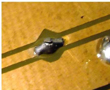
Figure 6. A good solder connection is a bright silvery cone
