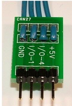
**Figure 9. The completed 4-pin Easy Connector.**
