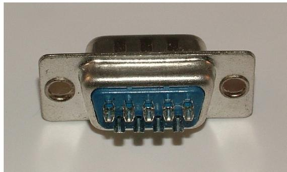
**Figure 3. The back of a DB-9 connector and its solder cups.**
