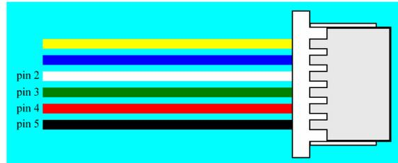
**Figure 2. Pin out of the six wire connector.**
