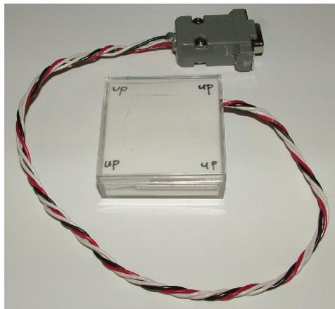
**Figure 11. The GT-320 is now buried inside the Lucite box and immobilized with neoprene foam.**
