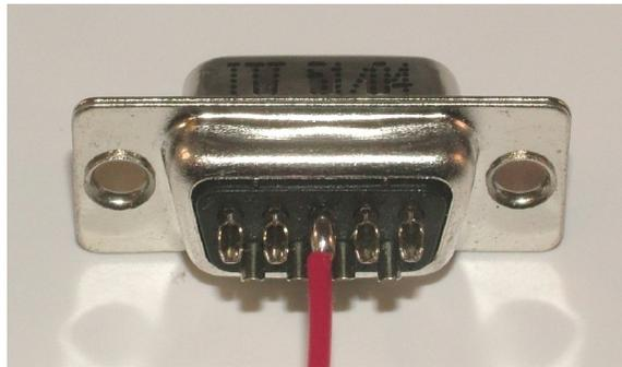
**Figure 4. The back of a DB-9 with a wire soldered to cup #3.**
