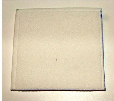
**Figure 6.** After pressing the Lucite box into neoprene, you can faintly see the box's outline.
