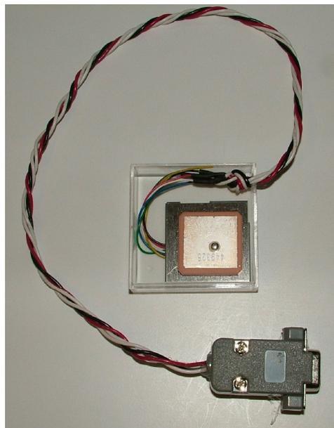
**Figure 9. The GT-320 inside the Lucite box. The knot in the GPS cable is too large to pass through the notch in the Lucite box.**
