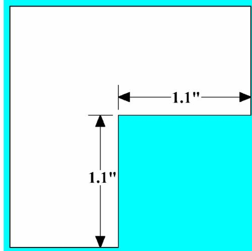
**Figure 8. The square notch cut into the thicker neoprene will prevent the GT-320 from sliding around inside the Lucite box.**
