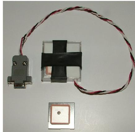
**Figure 1. The GT-320 GPS, in and out of its case.**
