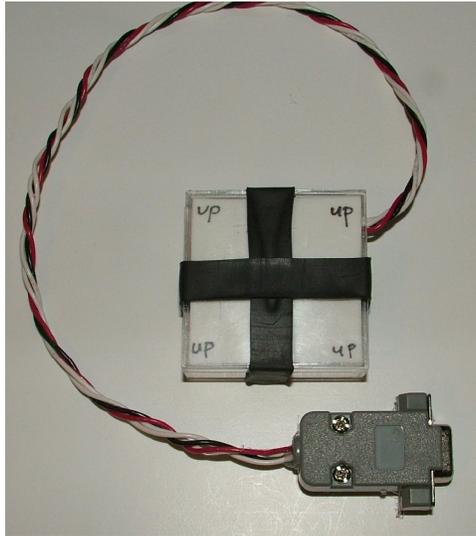
**Figure 12. The shrunken bands will keep the lid in place, but can be easily cut away to access the GT-320.**
